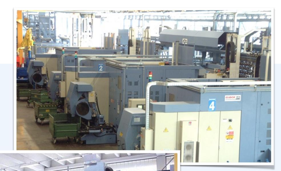
SMIMEC industrial plant is equipped with 20 CNC machining centers including 15 connected in FMS line that are able to carry out specific production programs even in the absence of operators.
